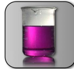
PURPLE - verified that the system is clean
